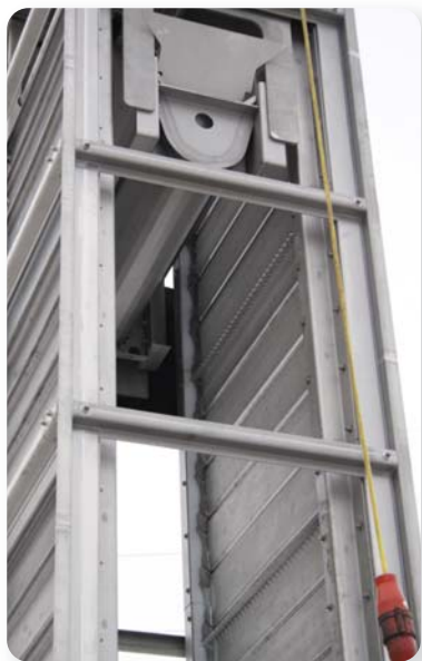
Solids are collected just below the discharge point at the apex of the filter belt.
