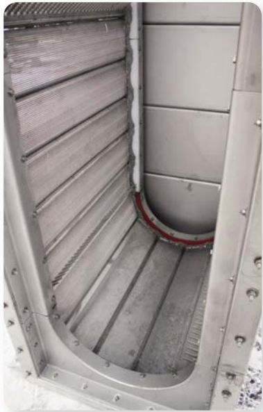
Special side seals on the frame prevent by pass.
